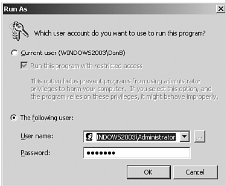
FIGURE 2.10 Running a program as a different user with the Run As right-click menu option.
