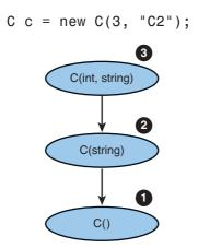
FIGURE 3.7 Constructor chaining sequence
