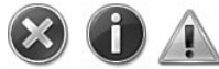
FIGURE 3.16 Standard icons for errors, information, and warnings need to be used for the corresponding status.
