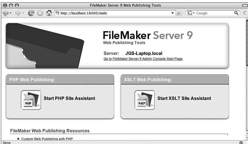
FIGURE 5.16 Click the Start PHP Site Assistant link on the Web Publishing Tools page to download and launch the PHPSA.
