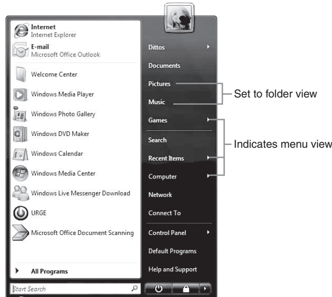
FIGURE 3.7 You can change the Start menu's right pane to display submenus or to open the submenu's contents in a folder view when you select the entry.
