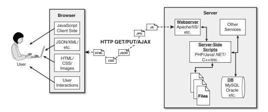
Figure 1.1 Basic diagram of the components of a basic website/web application.
