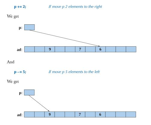
Using +, -, +=, and -= to move pointers around is called *pointer arithmetic*. Obviously, if we do that, we have to take great care to ensure that the result is not a pointer to memory outside the array:
