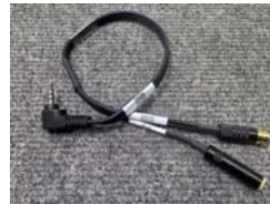
FIGURE 4.13 Mini TRRS-to-mini mic jack and mini headphone monitor jack for mobile devices
