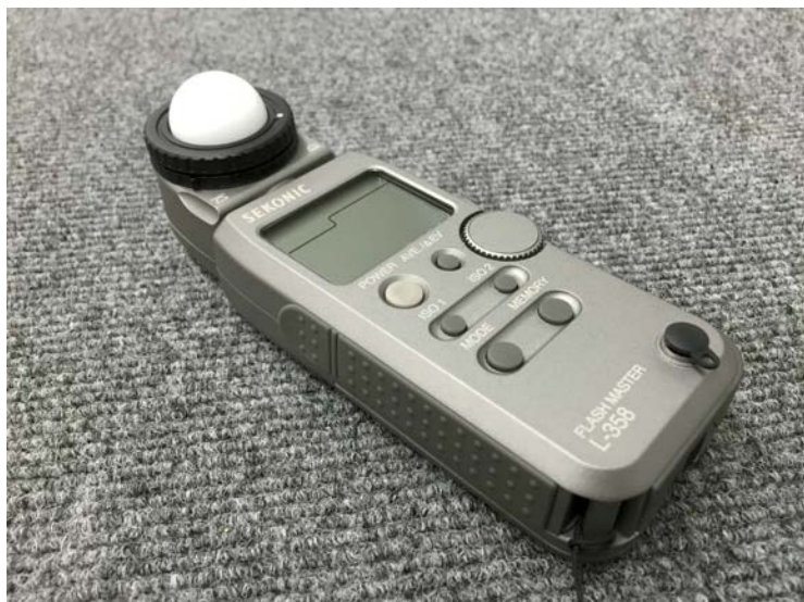
FIGURE 4.26 A digital light meter capable of incident and reflected light metering
