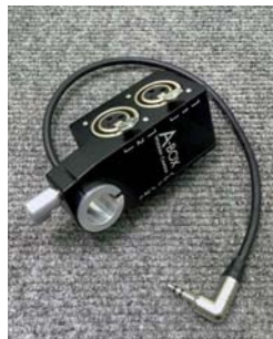
FIGURE 4.12 Wooden Camera A-Box mini TRS male to dual XLR female adapter box for DSLR camera rigs
