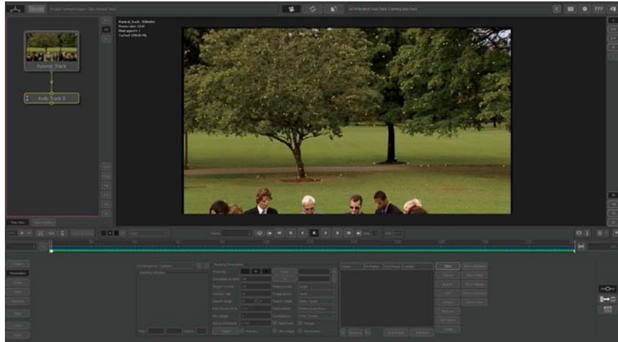
[Figure 4.30] The first step in a 3D track is a mass, automated 2D track.
