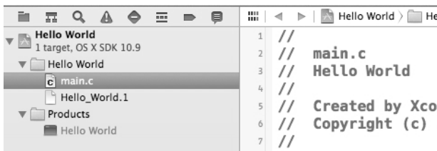
Figure 2.5 Clicking the name of an editable file in the Project navigator displays its contents in the Editor area.
