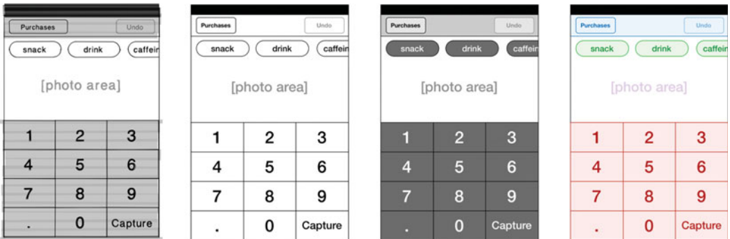
Figure 4.5 Several wireframing styles. Left to right: slightly sketchy, with the precise dimensions not yet nailed down; bare wires, to avoid suggesting any visual treatments; shaded, for suggesting relative visual weight; color-coded, for easy recognition of groups of elements.
