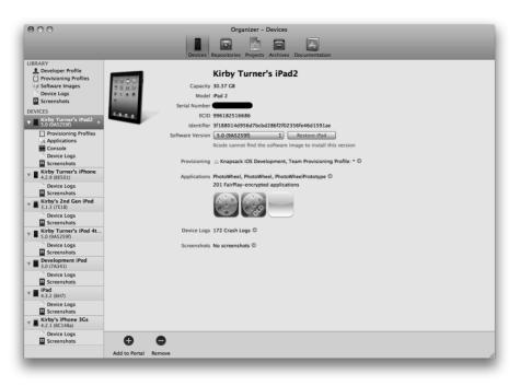
Figure 6.10 Organizer window with an attached Apple device ready for development
