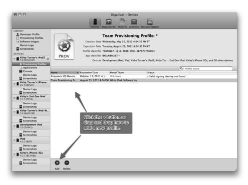
Figure 6.19 Click the + button or drag and drop the *.mobileprovision* file to add the development provisioning profile.
