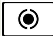
FIGURE 6.5 The Center-Weighted metering mode looks at the entire frame but emphasizes the center of it.
