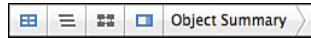
FIGURE 26.5 The Detail View buttons, which appear below the table portion of the Detail View. The first three buttons select different table displays, or “modes.” The modes are Table, Outline, and Diagram. The fourth button, showing a window with a portion on the right highlighted, opens or closes the Extended Detail pane. The Navigation Path breadcrumb control enables you to back a display off after you’ve drilled down into a detail.
