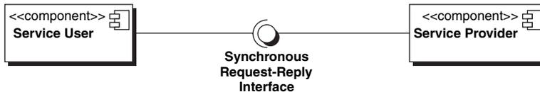
**Figure 4-2:** *Synchronous Request-Reply Interface*
