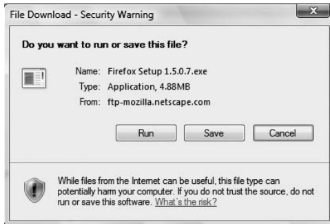
Figure 6.5 The Save option is safer because you can scan the downloaded file for viruses if you don't trust the website. It also leaves a copy of the program on your hard disk if you have to reinstall.
