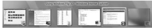
Figure 6.13 Alt-tabbing pops up a list of icons representing open windows. If you're using the Aero color scheme, the icons are live previews. Hold down Alt and press Tab repeatedly to highlight a window. If you press and release Alt+Tab quickly, you swap between only two windows instead of cycling through them all.
