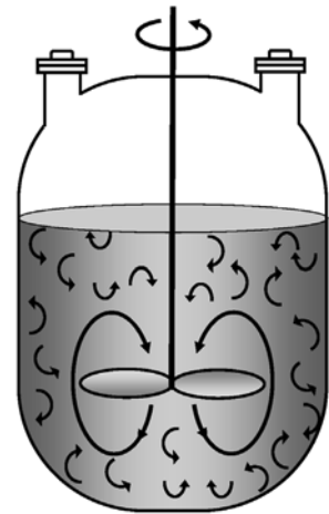
Figure 1-5(b) Batch reactor mixing patterns. Further descriptions and photos of the batch reactors can be found in both the Visual Encyclopedia of Equipment and in the Professional Reference Shelf on the DVD-ROM.
