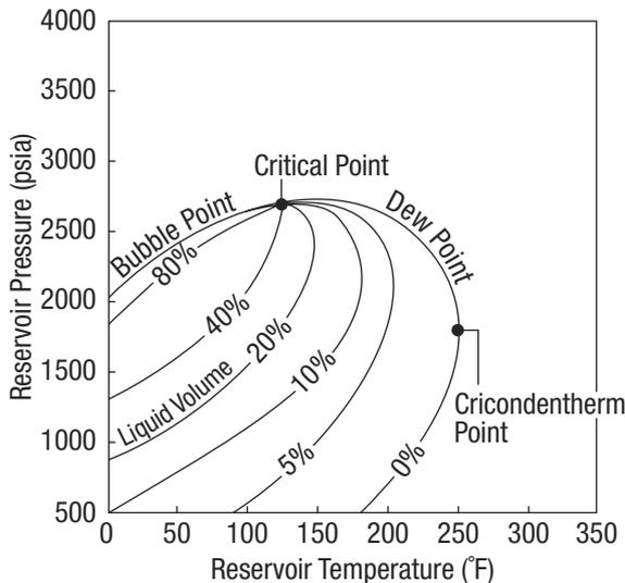
**Figure 1-3** Oilfield hydrocarbon phase diagram showing bubble-point and dew-point curves, lines of constant-phase distribution, region of retrograde condensation, and the critical and cricondenthem points.
