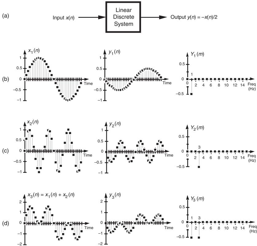
**Figure 1-7** Linear system input-to-output relationships: (a) system block diagram where  $y(n) = -x(n)/2$ ; (b) system input and output with a 1 Hz sinewave applied; (c) with a 3 Hz sinewave applied; (d) with the sum of 1 Hz and 3 Hz sinewaves applied.
