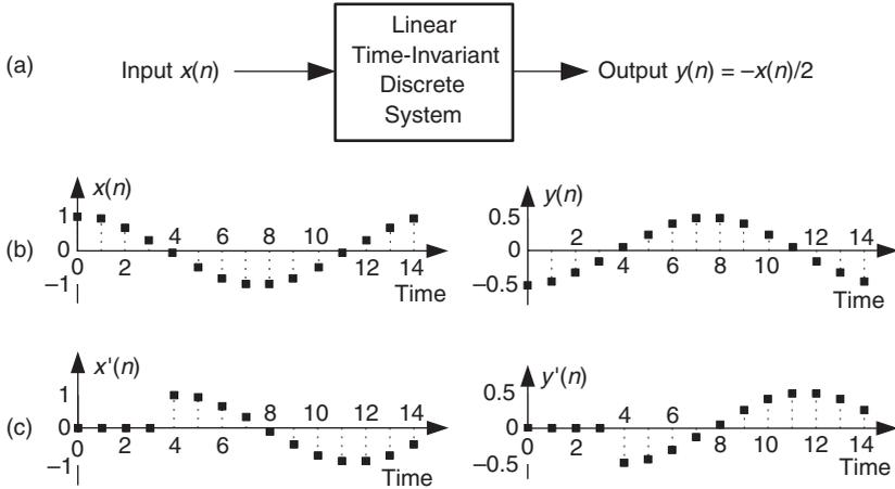
**Figure 1-9** Time-invariant system input/output relationships: (a) system block diagram,  $y(n) = -x(n)/2$ ; (b) system input/output with a sinewave input; (c) input/output when a sinewave, delayed by four samples, is the input.
