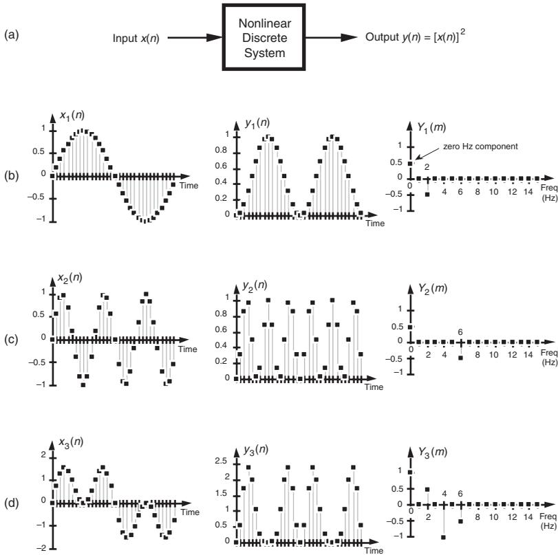
**Figure 1-8** Nonlinear system input-to-output relationships: (a) system block diagram where  $y(n) = (x(n))^2$ ; (b) system input and output with a 1 Hz sinewave applied; (c) with a 3 Hz sinewave applied; (d) with the sum of 1 Hz and 3 Hz sinewaves applied.
