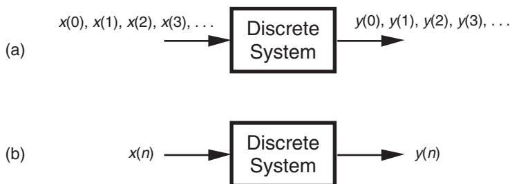
**Figure 1-2** With an input applied, a discrete system provides an output: (a) the input and output are sequences of individual values; (b) input and output using the abbreviated notation of  $x(n)$  and  $y(n)$ .
