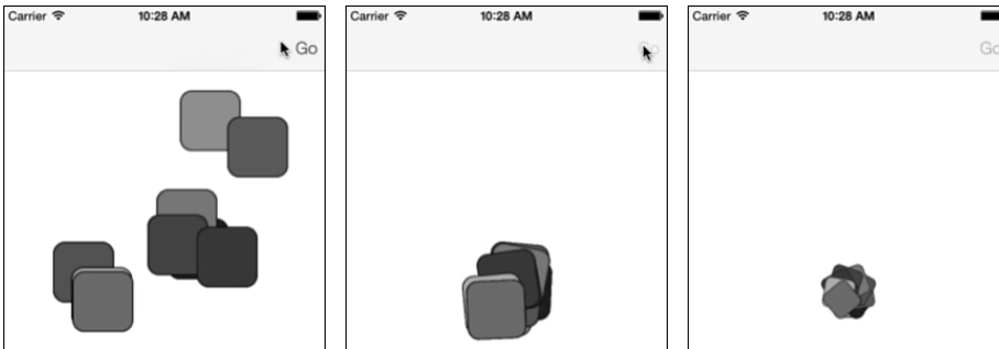
Figure 6-2 In this animation, a snap behavior draws the views together, and a transformation behavior angles each item to form a tight nest.
