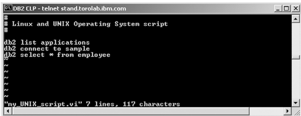
Figure 4.10 Invoking DB2 CLP commands and SQL statements in a Linux/UNIX script file
