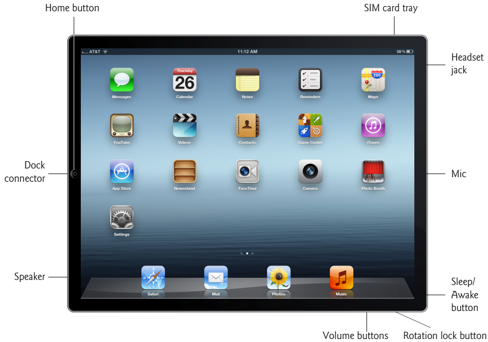
Fig. 1.3 | iPad hardware—all but the Home button are on the side or back of the device.
