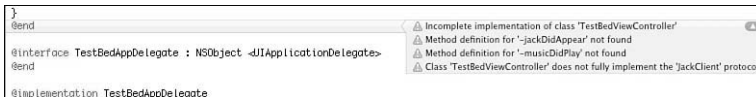
Figure 3-3 You must implement all required methods to conform to a protocol. Objective-C warns about incomplete implementations.
