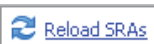
Figure 9.17 With the Reload SRAs link, the SRM administrator doesn't have to restart the core vmware-dr service for changes to take effect.
