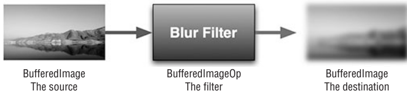
Figure 8-2 Filtering an image with Java 2D.
