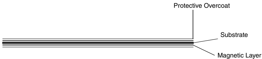
Figure 4-1 Material Layers in a Disk Media Platter
