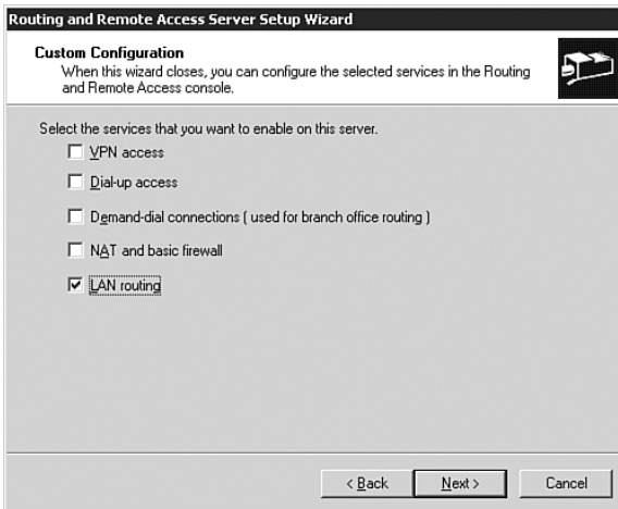
FIGURE 2.27 The LAN routing option is the bare minimum you need to support later installation of the DHCP relay agent.
