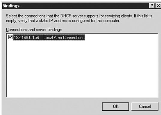
FIGURE 2.40 You can view and change the DHCP bindings from the Bindings window.
