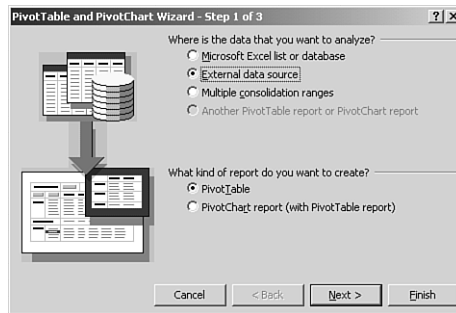
Figure 30.7 OLAP data access starts with the PivotTable and PivotChart Wizard. OLAP server data is defined as an external data source.
