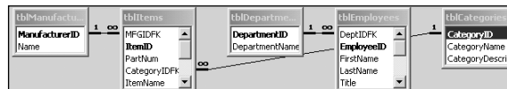
Figure 4.2 You can use Microsoft Access's Relationship feature to view a graphical representation of the relationships between tables. Notice that the links connect primary keys to foreign keys.
