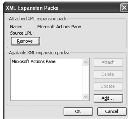
FIGURE 15.12: The ActionsPane solution attached to an Excel workbook is visible in Excel's XML Expansion Packs dialog box and can be removed if ActionsPane.AutoRecover is not set to True .
