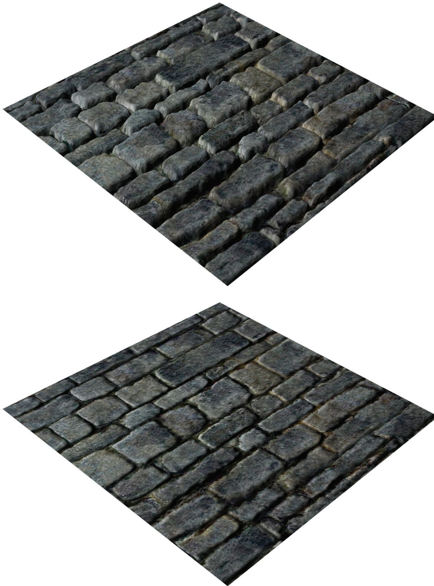
Figure 8-1. A Displaced Stone Surface Displacement mapping (top) gives an illusion of depth not possible with bump mapping alone (bottom).
