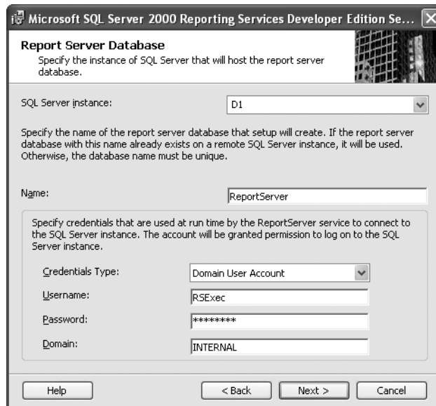
Figure 2.4 Select the Report Server Database and the Domain Account That Accesses It
