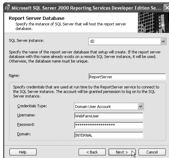
Figure 2.13 “D2” Is a Secondary Development Server Where Reporting Services Was Already Installed. This Screen Was Captured While Executing Setup on Server “D1”
