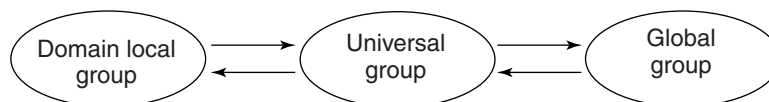
Figure 3.31 You can change a group scope to and from a universal group, but you can't change scope directly from a domain local group to a global group or vice versa.
