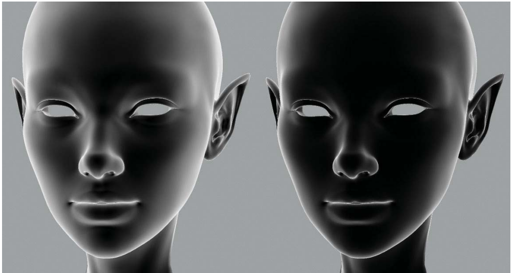
Figure 3-7. Dot Products Stored in SkinSilhouetteVec On the left, (1 - (\mathbf{N} \cdot \mathbf{V})) ; on the right, (1 - (\mathbf{N} \cdot \mathbf{V}))^2 .
