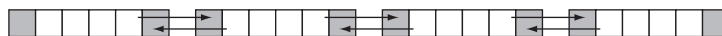
Figure 4.10: A data distribution with ghost boundaries. Shaded cells are ghost copies; arrows point from primary copies to corresponding secondary copies.
