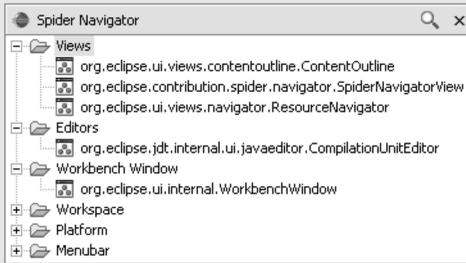
Double clicking an object in the Spider Navigator adds it to the Spider drawing.
