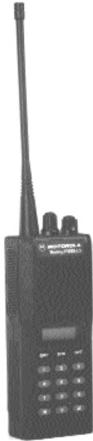
Figure 1.4, Traditional Land Mobile Radio Source: Motorola
