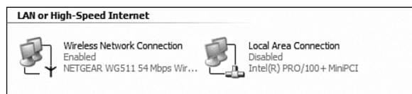
**FIGURE 10-11** Disabling the unused wired connection.
