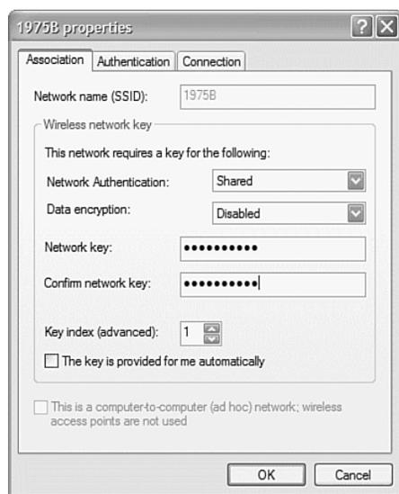
**FIGURE 10-9** Entering a network key for authentication.
