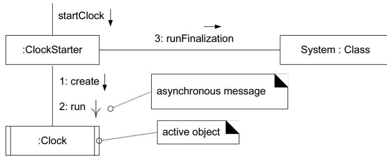
Figure 15.35 Asynchronous call in a communication diagram.
