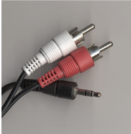
FIGURE 3.10 Some components, such as computer sound cards, use a 3.5mm mini-stereo plug for audio. You can use an adapter like this one to connect to a miniplug jack.
