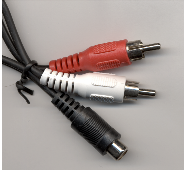
FIGURE 3.8 A Y-shaped adapter will let you feed a monaural signal to a stereo input, or send a stereo signal to a device that accepts only monaural input.
