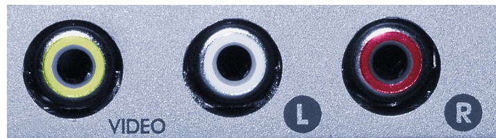
FIGURE 3.7 Composite video/audio use three RCA jacks color-coded yellow, red, and white.
