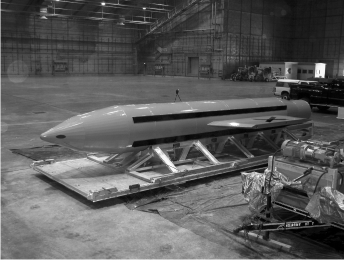
Figure 3–4 Massive Ordnance Air Blast weapon is prepared for testing at the Eglin Air Force Armament Center. (Source: DefenseLink)
