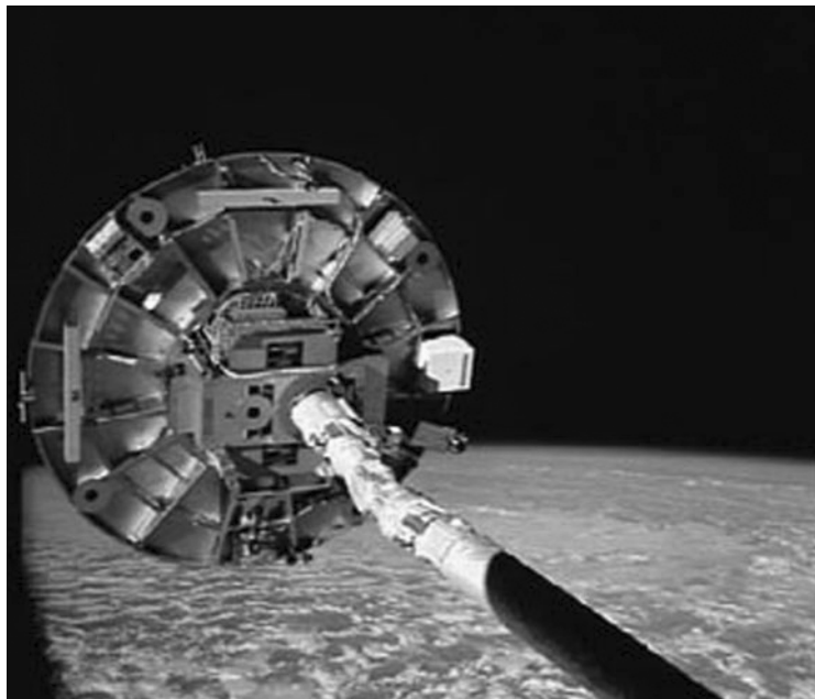
Figure 9.2 The Wake Shield Facility being held out in space by the shuttle's robot arm. Image courtesy NASA.
