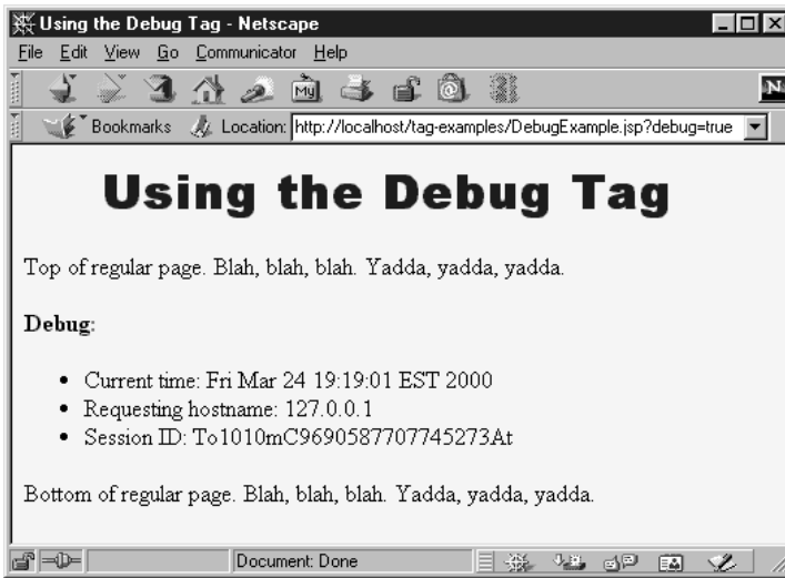
Figure 14-6 The body of the csajsp:debug element is included when a debug request parameter is supplied.
