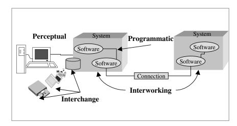
FIGURE 3.10 Conformance Reference Points for Testing
