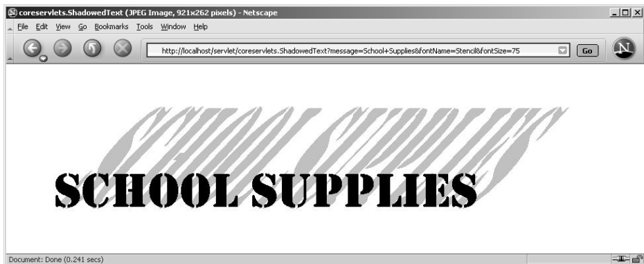
Figure 7-8 One possible result of the image-generation servlet. The client can save the image to disk as somename.jpg and use it in Web pages or other applications.
