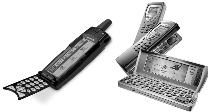
FIGURE 5–6 PDA/phone hybrids powered by EPOC. Left image courtesy Sony Ericsson Mobile Communications. Right image courtesy Nokia.
